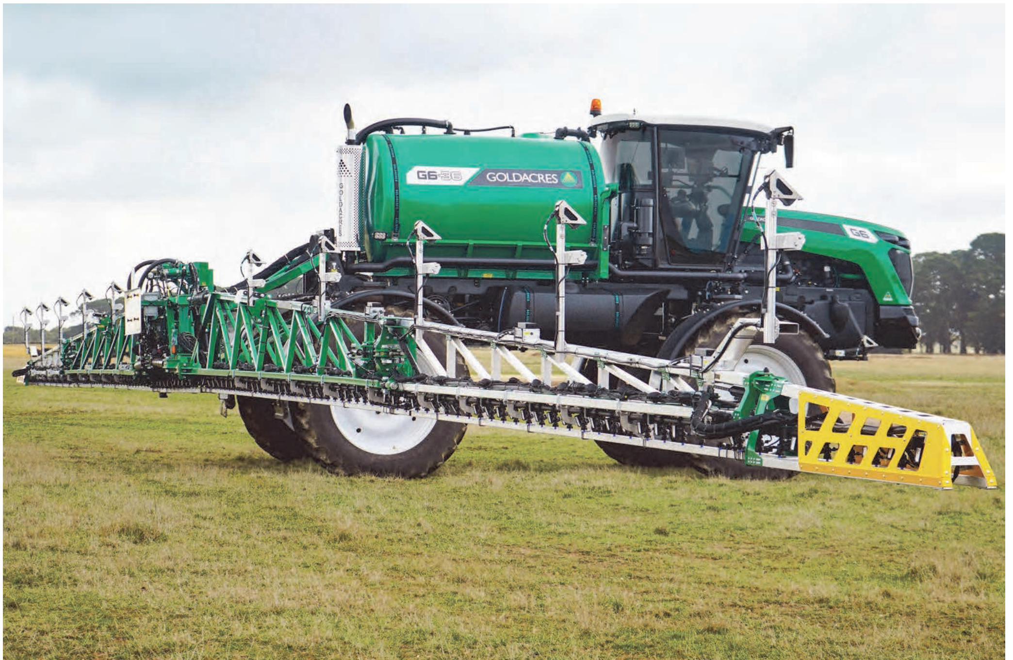
The Goldacres G6 Crop Cruiser Series 2 fitted with AI precision spraying technology Weedetect.
