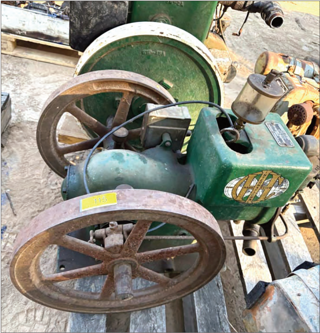
• Lot 115, International harvester stationary engine no. bx2884. speed 600. 3hp. In running condition.
