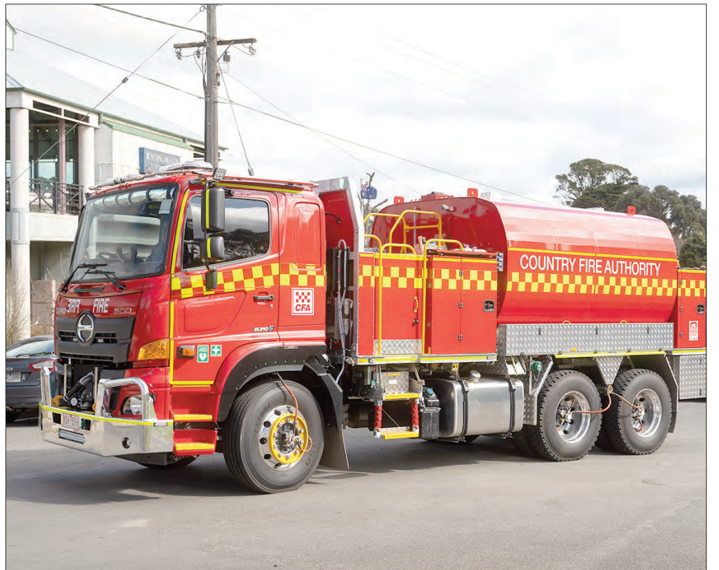
• The Ultra heavy tanker is the most recent truck to join the fleet, capable of carrying 10,000 litres of water.
